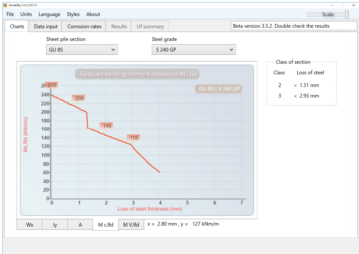
Figure 5.4 Results from the Durability tool for a GU 8S with a steel grade S 240 GP [ArcelorMittal]
