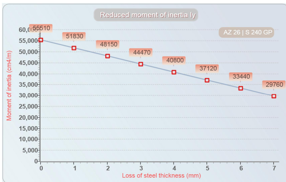
Figure 3.7 For loss of steel thickness reduced moment of inertia of a AZ26 S240GP by [ArcelorMittal, 2017]
